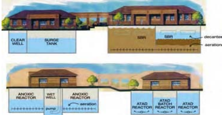
Water Reclamation Facility's Underground Treatment Process
