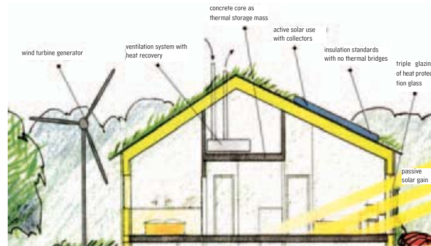
Principle of a 'Lummerland' passive house
